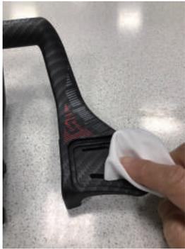
① Cleanse the contact surface between elbow pad and chassis.
