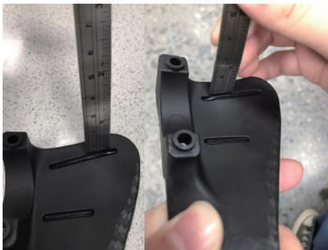
⑤ Use steel ruler or similar tool to needle-pick the rib of the elbow pad to ensure the elbow pad is thoroughly installed.
