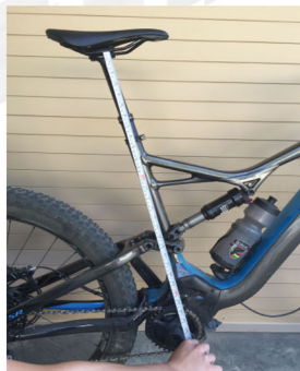
Measure height to saddle rails, record measurement This will be used later after cable installation
